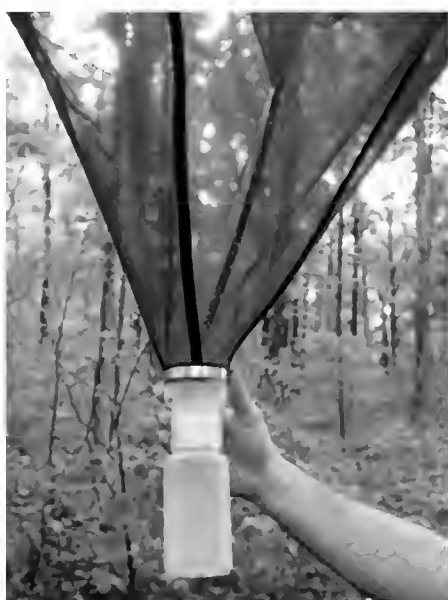
(figure 2.) Lower collection vial where beetles that “hit and drop” are collected.
